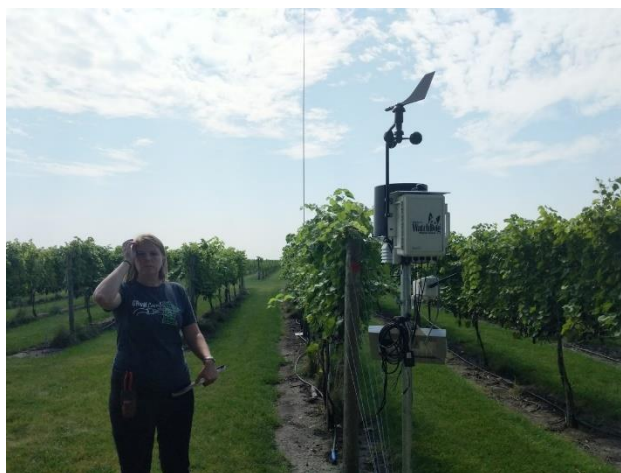
A wireless distress call speaker in a vineyard, mounted to a weather station. Photo: Davy DeKrey.
